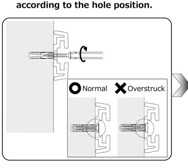
②Drill the holes (Diameter 5 mm, depth 35 mm)
