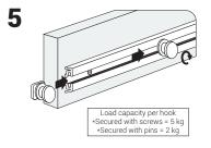
Slide the hook through and turn clockwise to secure.
