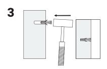
Install the anchor into the hole.
