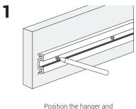
Position the hanger and mark the hole positions.
