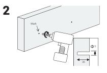
Drill the holes. (Diameter 5 mm, depth 35 mm)
