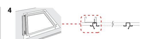
Insert TENKENKO-T, with the beam attached, into the opening and use the beam to hold the frame within the opening.
