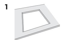
Cut an opening in the ceiling board to the appropriate size. **450** - 500x500mm **600** - 650x650mm
