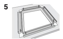
Attach a beam to each remaining side with 2 screws, for a total of 4 beams and 8 screws.
