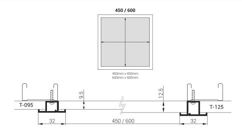
Note: The 2 sizes (450 & 600) are available in 2 different configurations, 1 for use with 9.5mm board and 1 for use with 12.5mm board.
